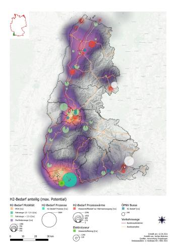
Fig. 5.4: Heat map for projected hydrogen demand on the German side as well as the list for the hydrogen use in 2021 (H<sub>2</sub>-SO: Wasserstofftechnologien am Südlichen Oberrhein Potentialerhebung –Räumliche Analyse Klimapartner Oberrhein 2021).
