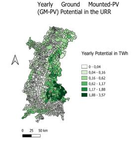
Fig. 3.7: The technical potential of GM-PV per municipality of the Upper Rhine Region (Najjar et al., 2022, 24).
