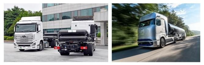
Fig. 5.21: left: XCIENT fuel cell truck (Hyundai); right: GenH, with LH, tanks of Daimler Trucks (Daimler Trucks)
