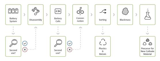
Figure 4.8: Approach of dismantlement and recycling of aged electric vehicle batteries including diagnostics
