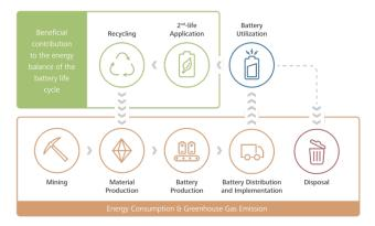
Fig. 4.1: Lifecycle of a battery (Dühnen et al., 2020: 3).
