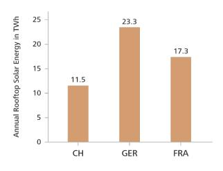
Fig. 3.3: Rooftop Solar PV potential in the Upper Rhine Region in TWh/y (Najjar et al., 2022, 22).
