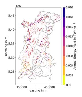
Fig. 3.2: Distribution of technical potential for wind energy on the usable area in the Upper Rhine in TWh per year (Najjar et al., 2022, 21)
