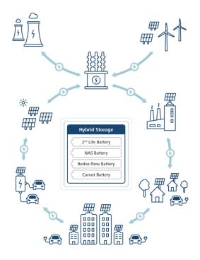
Fig. 4.6: Concept of grid-scale / large-scale hybrid EES consisting of second-life LIBs, a NAS battery, a vanadium redox-flow battery and a Carnot battery (edited from Gattiglio, 2017)
