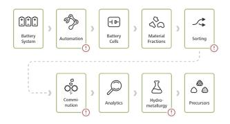
Fig. 4.9: Process steps in the disassembly and recycling process that will be further developed for the planned pilot projects
