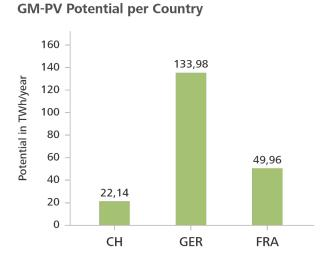
Fig. 3.5: Preliminary technical potential of GM-PV in the Upper Rhine Region (Najjar et al., 2022, 24).
