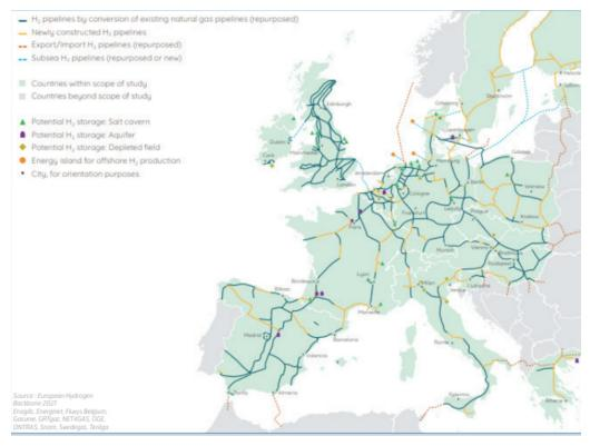
Fig. 5.10: Planned European Hydrogen Backbone⁵ (Guidehouse, 2020)
